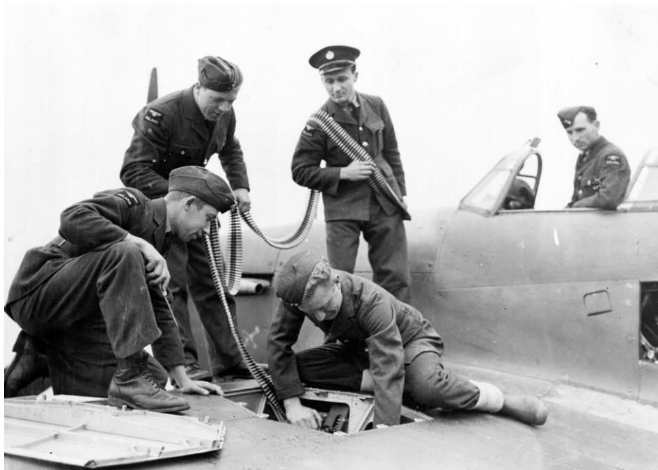
Armourers replenish the guns of Hawker Hurricane I of 303 (Polish) Squadron at Leconfield, Yorkshire, 24 th October 1940.
